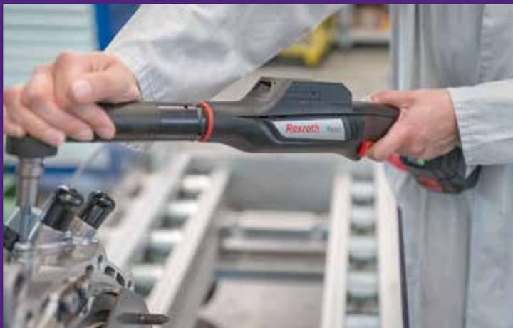
*On Bosch's Nexo nutrunner, the integrated control system enables wireless connectivity to higher-level systems.*
